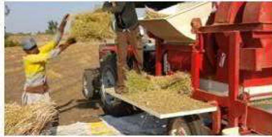
Picture 2: Tractor operated coriander threshing
